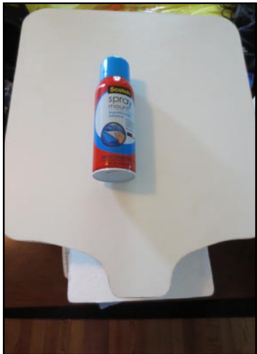
You have to secure a T-shirt to the platen; this process is very simple. Coat the platen with a thin coat of spray mount; it doesn't take a lot of spray.
