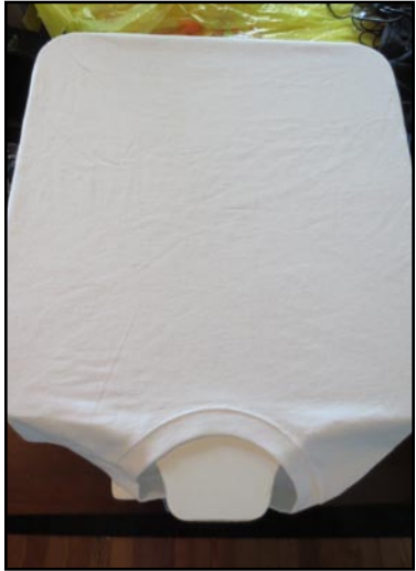
The main purpose of securing the T-shirt to the platen is so that it doesn't move during printing. If you are printing two or more colors, it is essential the shirt remains stable.
