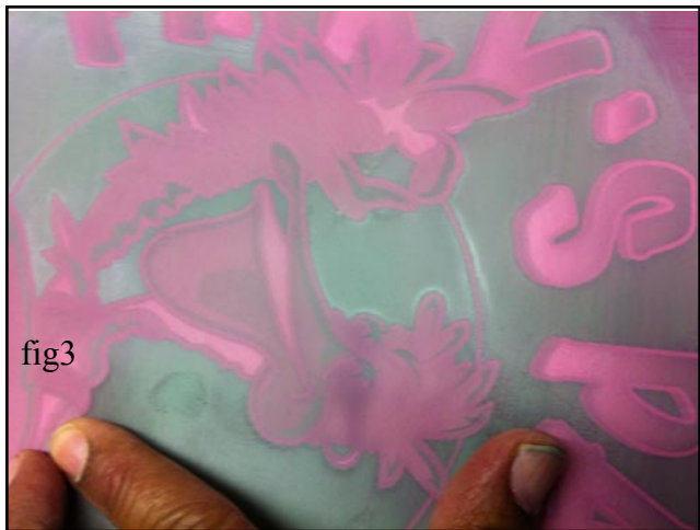
When setting up your screen for printing, remember a good technique is off contact printing. The screen should be installed about 1/2 inches above the platen. This gap insures a clean smooth layer of ink will be applied. The screen will stretch down, print the shirt, and return to its original position.
