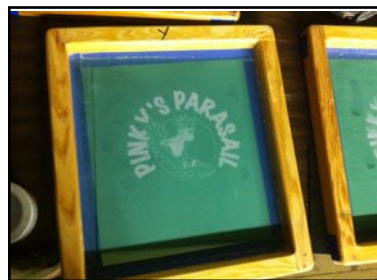
A very important step with the screens is that you have to tape them off. This means you have to tape any gaps in the screen that will allow ink to seep through. In this photo, the gaps are where the screen and wood frame meets.
